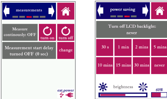
Left: measurement settings (measure continuously and start delay Right: power saving settings (backlight time-out and display brightness)
