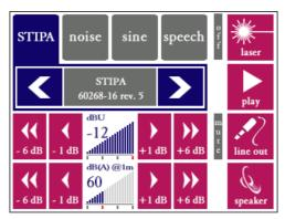
Select any of the tabs on the top-left bar to access any of the four categories of test signals: Speech intelligibility (STIPA), Noise, Sine or Speech. Then choose the test signal which you need for your measurements. Consult chapter 4 of this manual for further explanations on the different types of test signals.
