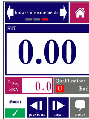
*“Settings” screen and “browse measurements” screen. The latter screen is nearly identical to the STI measurement screen, but with previous/back buttons instead of start/stop and save buttons.*
