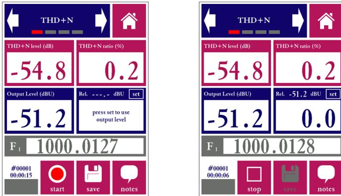
*Measuring screen before setting a reference level (left) and after setting the reference level in dB to 2.7 dB (right)*
