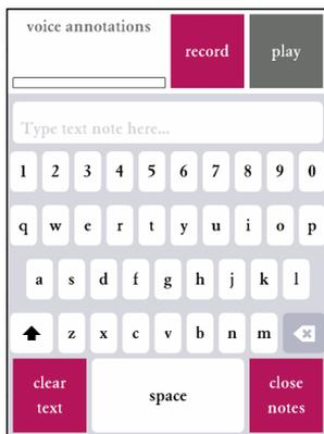
Text notes are saved in a text file (.TXT), voice notes in a .WAV file - each with the same serial number as the current measurement. Voice annotations can be recorded either through the measurement microphone or a headset microphone (connected through the headset jack on the side of the device). The input channel can be selected in the “Settings” module.
