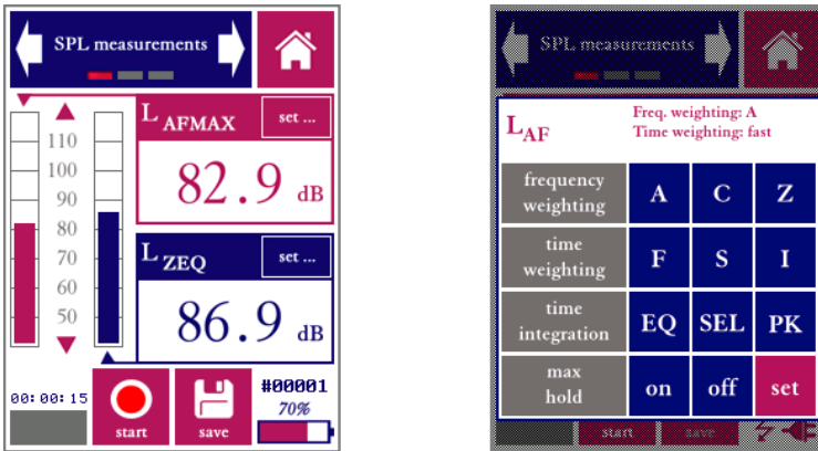
SPL measurements screen, during measurement (left) and with settings keyboard showing (right)
