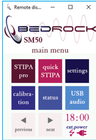
The main menu from the Bedrock SM50, as accessed through the Remote Display application under Windows 10.
